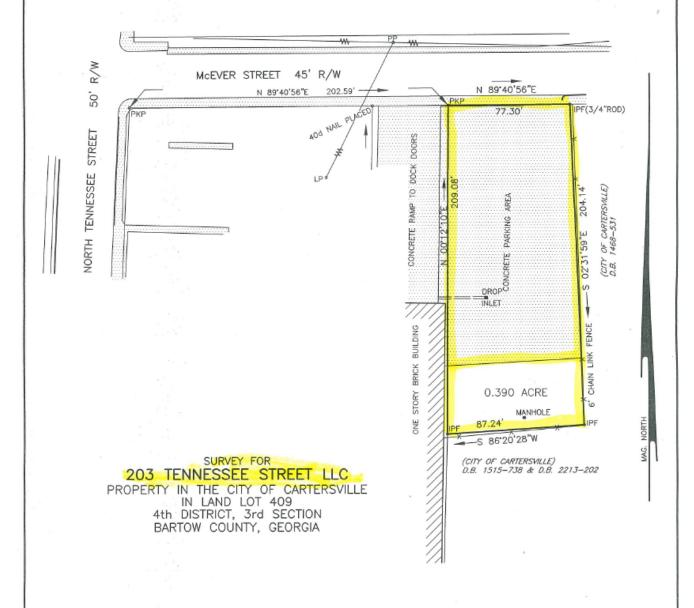
FIELD TRAVERSE: CLOSURE; ONE FOOT IN 20,000 FEET USING A LIETZ SET 3. ANGULAR ERROR; 0'00'06"PER ANGLE POINT USING A LIETZ SET 3. ADJUSTED; USING THE COMPASS RULE.
