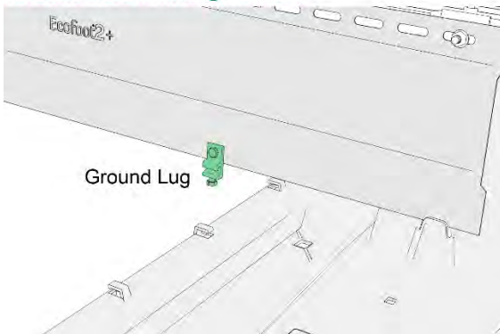
Ground hole with Lug Installed
