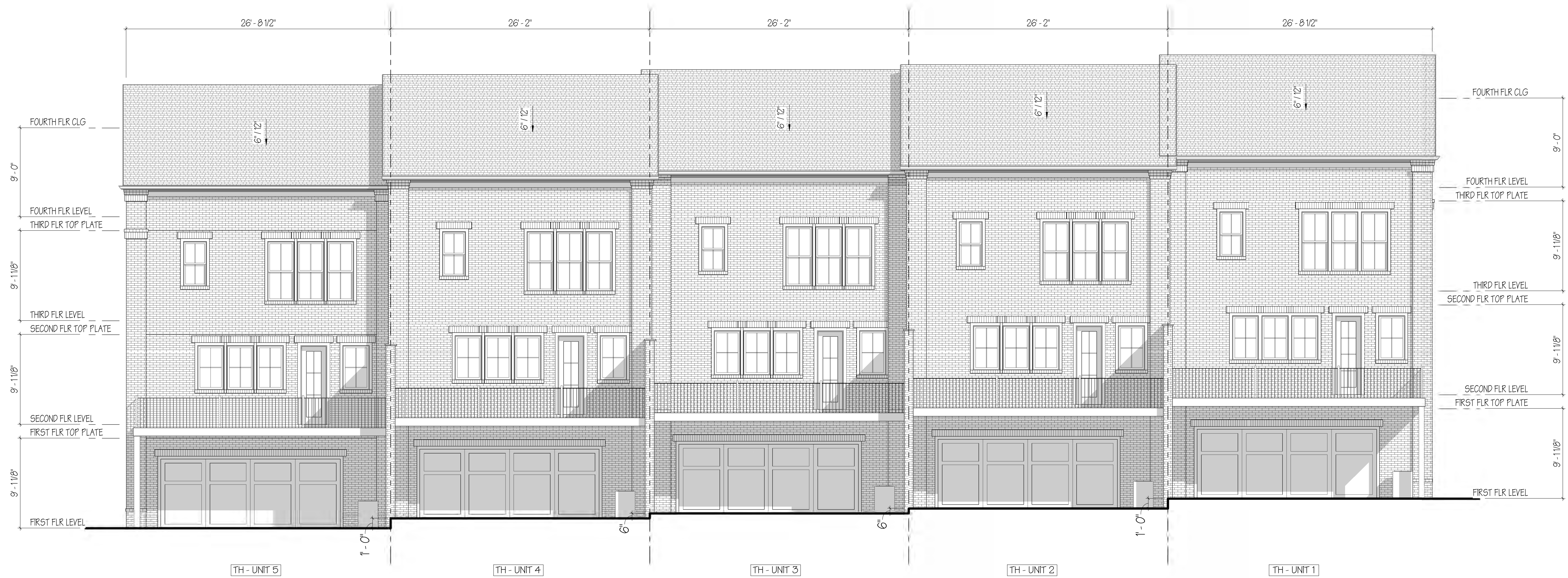
① BUILDING 1 - REAR ELEVATION 3/16" = 1'-0"
