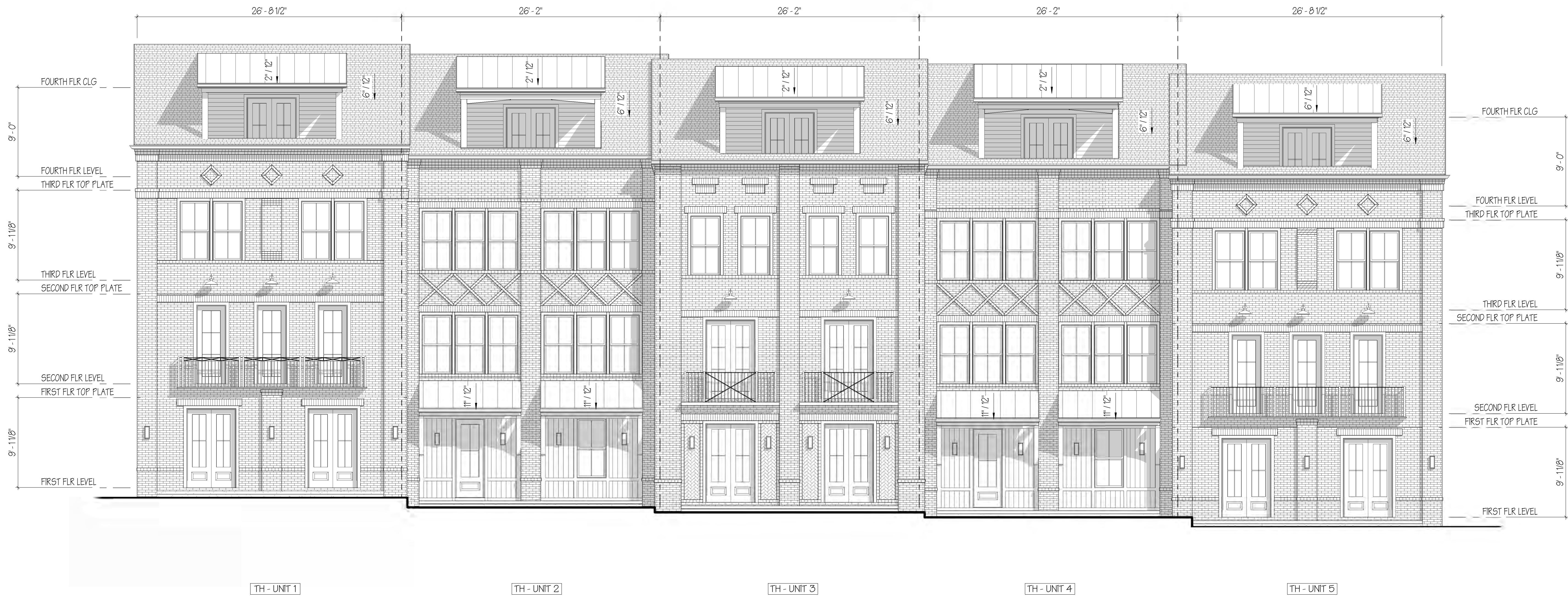
① BUILDING 1 - FRONT ELEVATION 3/16" = 1'-0"
