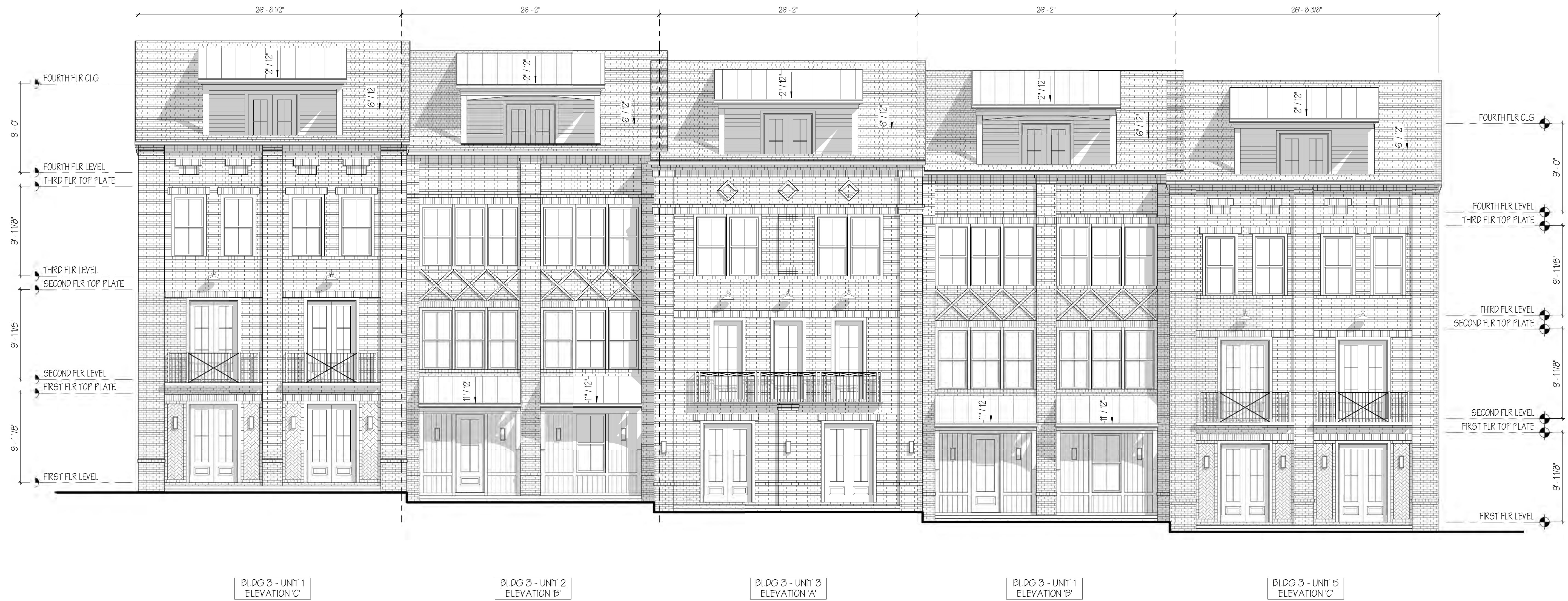
① BUILDING 3 - FRONT ELEVATION 3/16" = 1'-0"
