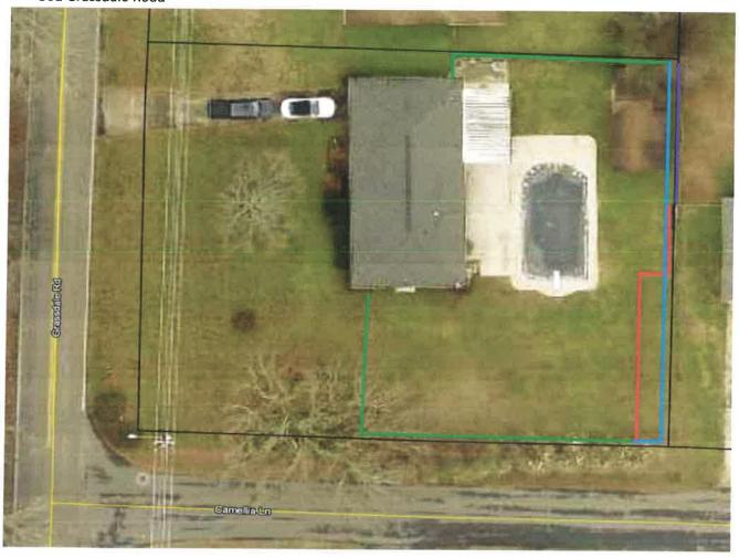
Existing chain link fence to be removed and replaced with 6' privacy fence
