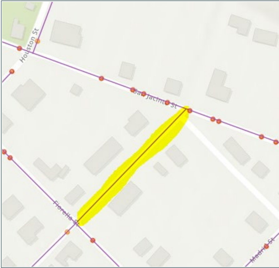
Figure 53: Petersburg St between Fiorella St and San Jacinto St (field verified as 1" steel)
