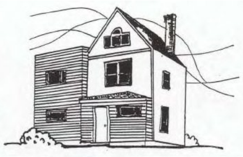
Even new construction and additions that use traditional materials (wood siding) in an inappropriate way fail to blend with the original
