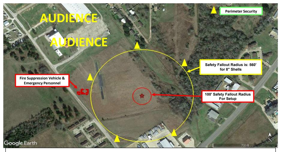
SECURED AREA A MINIMUM OF 560' FROM ALL SIDES OF THE FIRING SITE. NO SCHOOLS, CHURCHES, HOSPITALS, LICENSED CHILD CARE, HEALTH CARE, DETENTION, CORRECTIONAL FACILITY OR ASYLUMS WITHIN 600' FROM ALL SIDES OF THE FIRING SITE. NO HAZARDOUS MATERIALS WITHIN 1,120' FROM ALL SIDES OF THE FIRING SITE. PERIMETER SECURITY IS THE RESPONSIBILITY OF CITY OF CROCKETT.
