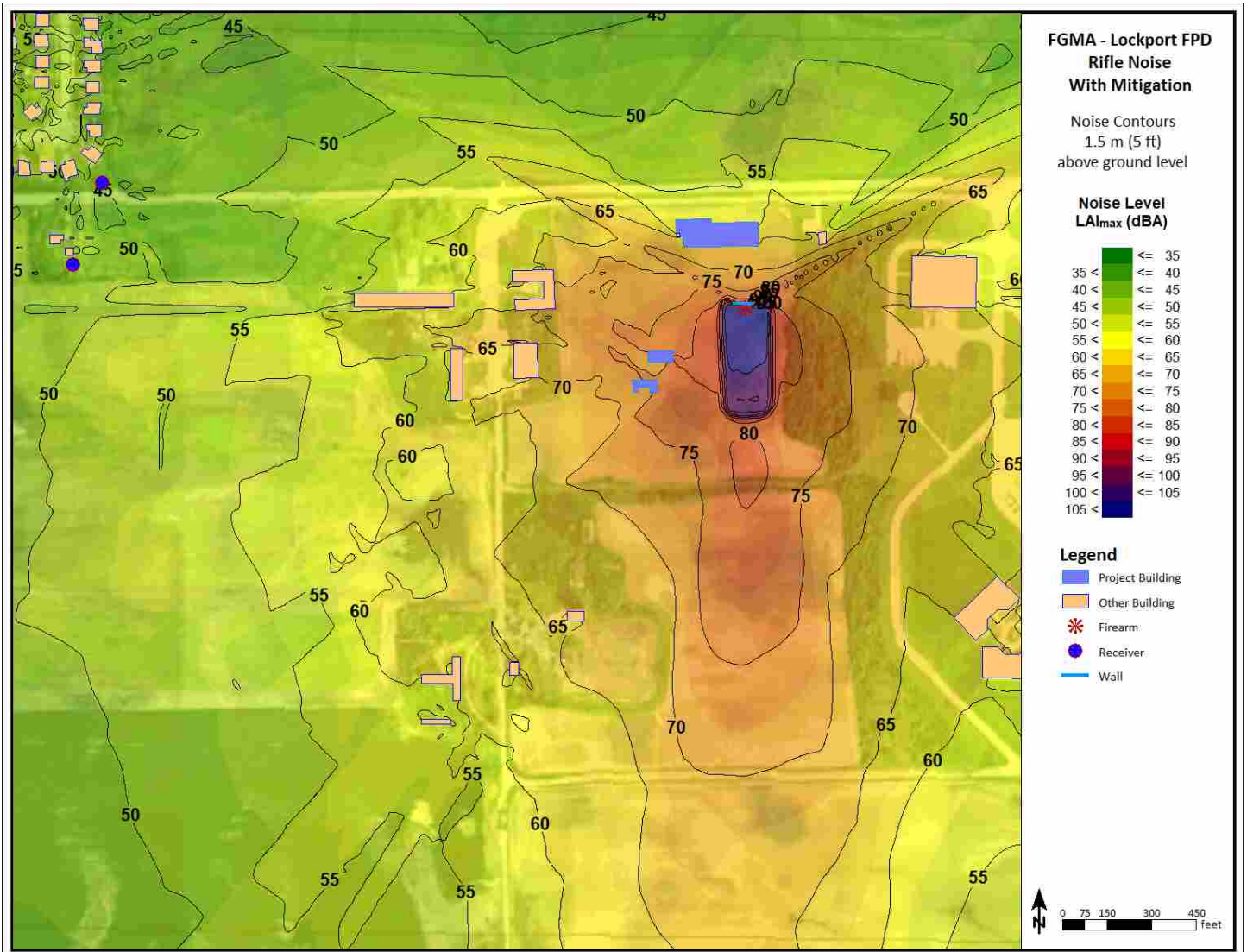
Figure 12: Noise Contour Map of Predicted Rifle Noise Transmission Near Project Site, With Berms and Barrier
