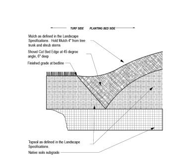
SPADED PLANTING BED EDGE DETAIL SCALE: NO SCALE
