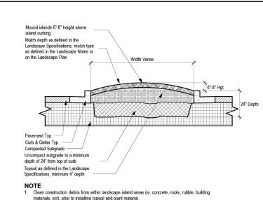
2. Fracture/nosen existing subgrade to a minimum 44\* deptin. Remove and replace any subgrade unsuitable for planting. Once subgrade is clean of debris and loosened, add topsoil to a minimum bermed 6\*-8\* height above island curbing.
