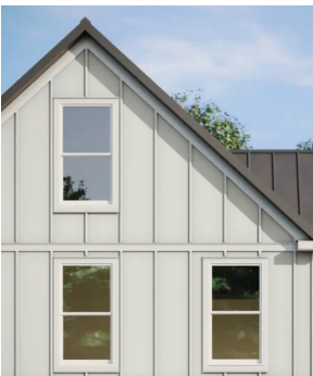
SIDING: JAMES HARDIE SMOOTH PANEL 10' X 4' SMOOTH BATTEN STRIPS 2.5" X 3/4" @ 12" O.C.
