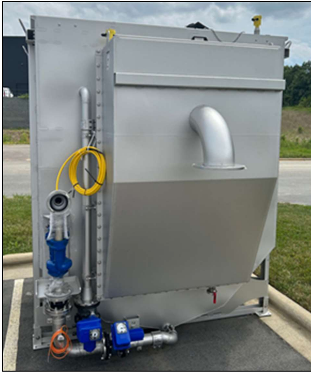
Effluent and backwash piping
