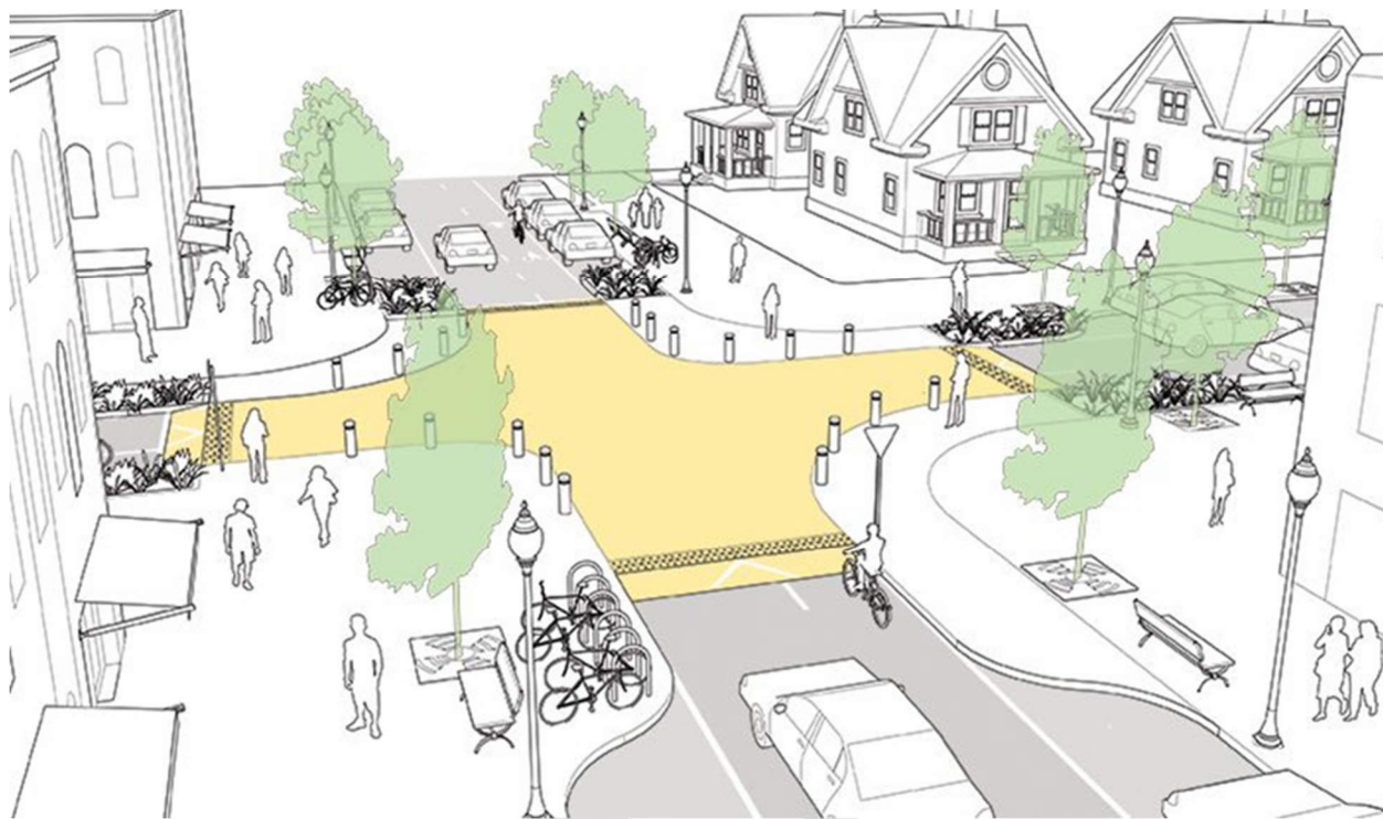
Figure 44 NACTO Raised Intersection.
