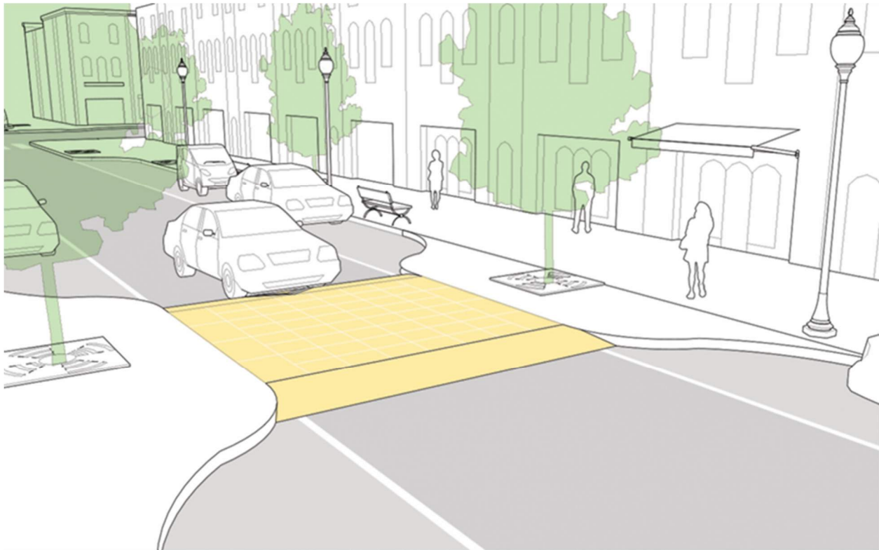
Figure 51 NACTO Speed Table.
