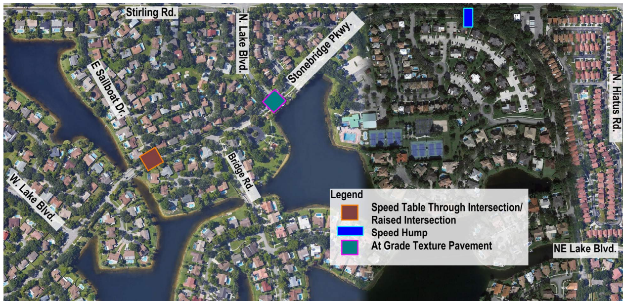
Figure 60 Stonebridge Pkwy. Proposed Location of Improvements
