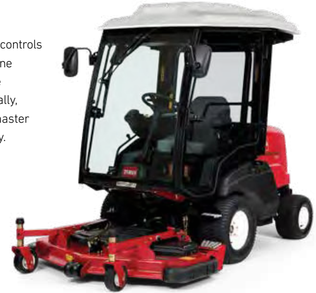
ALL-SEASON CAB All-season cab with heat and air conditioning is standard on model 3310. Optional heat-only cab (no air conditioning) for other models.
