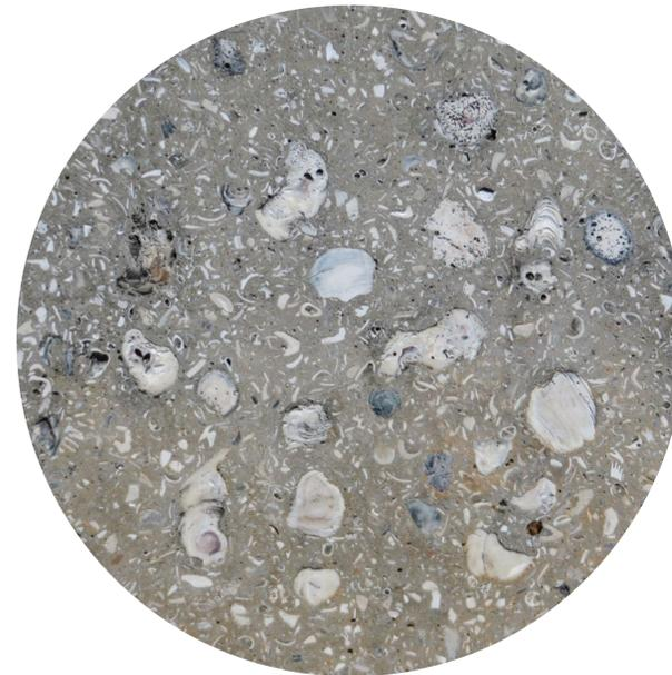
7. SHELLROCK AGGREGATE CONCRETE
