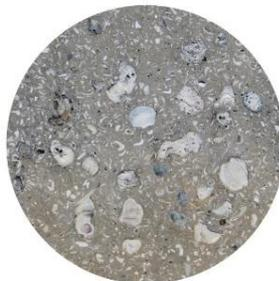
7. SHELLROCK AGGREGATE CONCRETE
