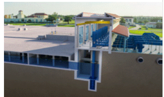
Figure 6.7. High Service Pump Station
