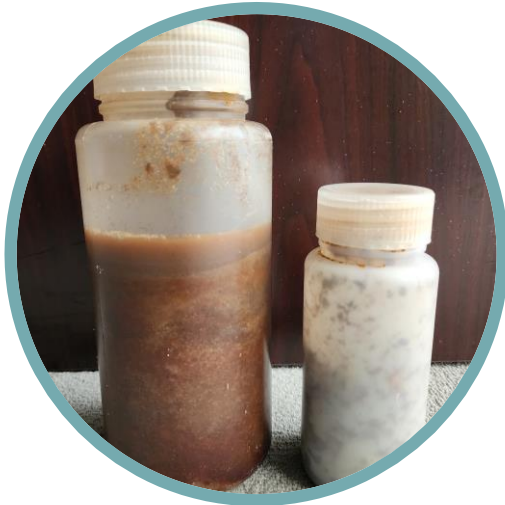
Iron scaling and sediment in raw water
