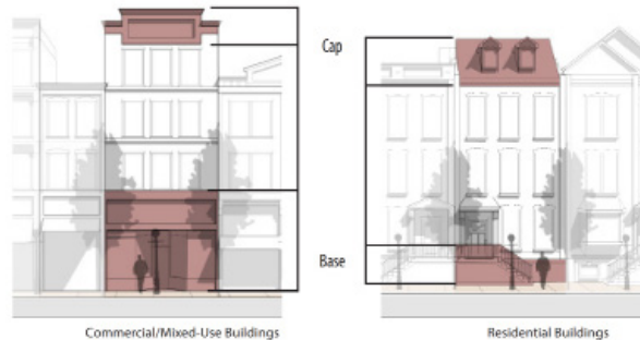
Figure 1.32: Building Base, Middle and Cap, Davidson, NC
