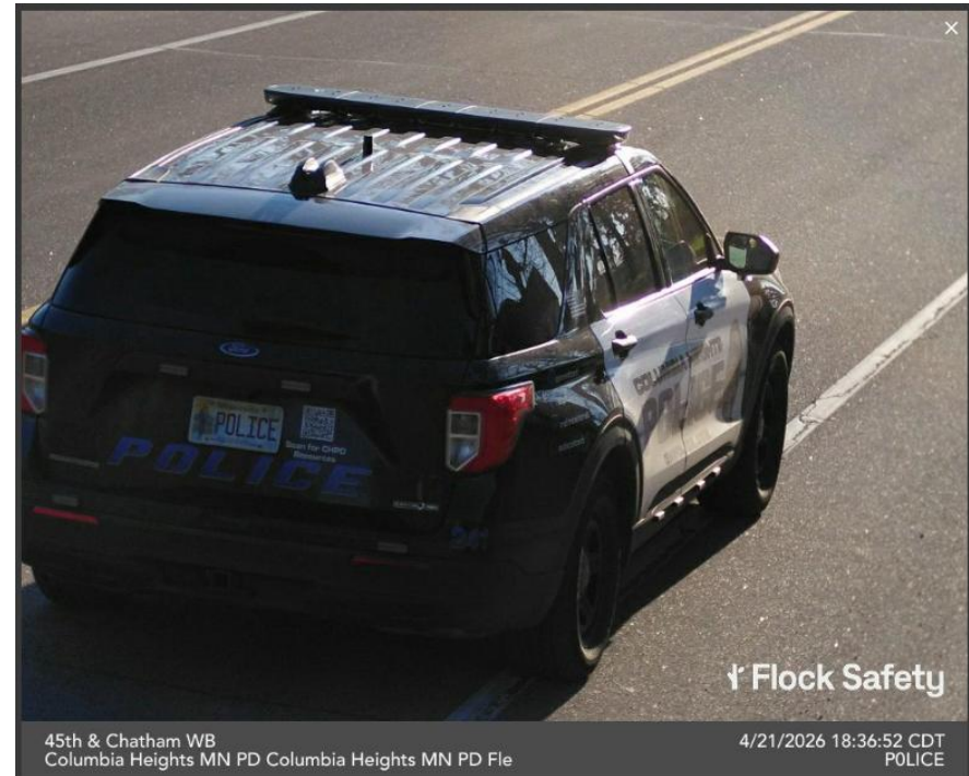
This is the angle required by Flock Cameras to view Plates and Vehicle data – Any higher and they would not capture anything.
