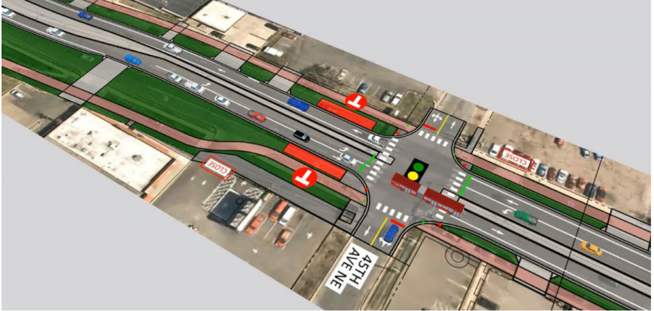
Figure 3 - Screen shot of traffic simulation of bus stopping in-lane at 45th Ave.
