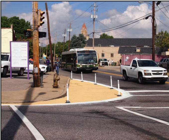
Low cost curb extension with paint and removable pylons
