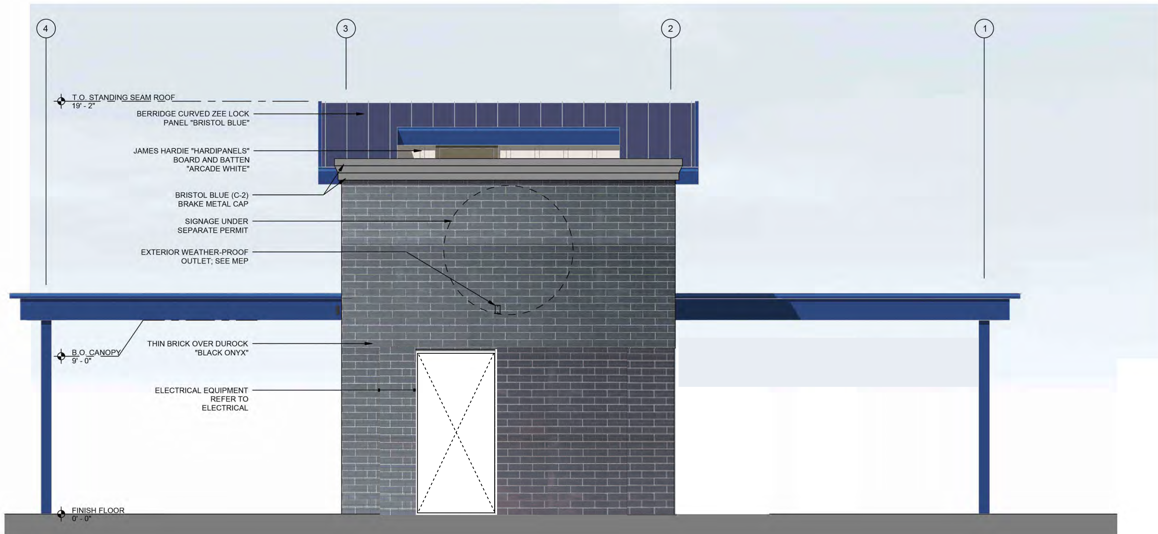
FACING WEST ELEVATION
