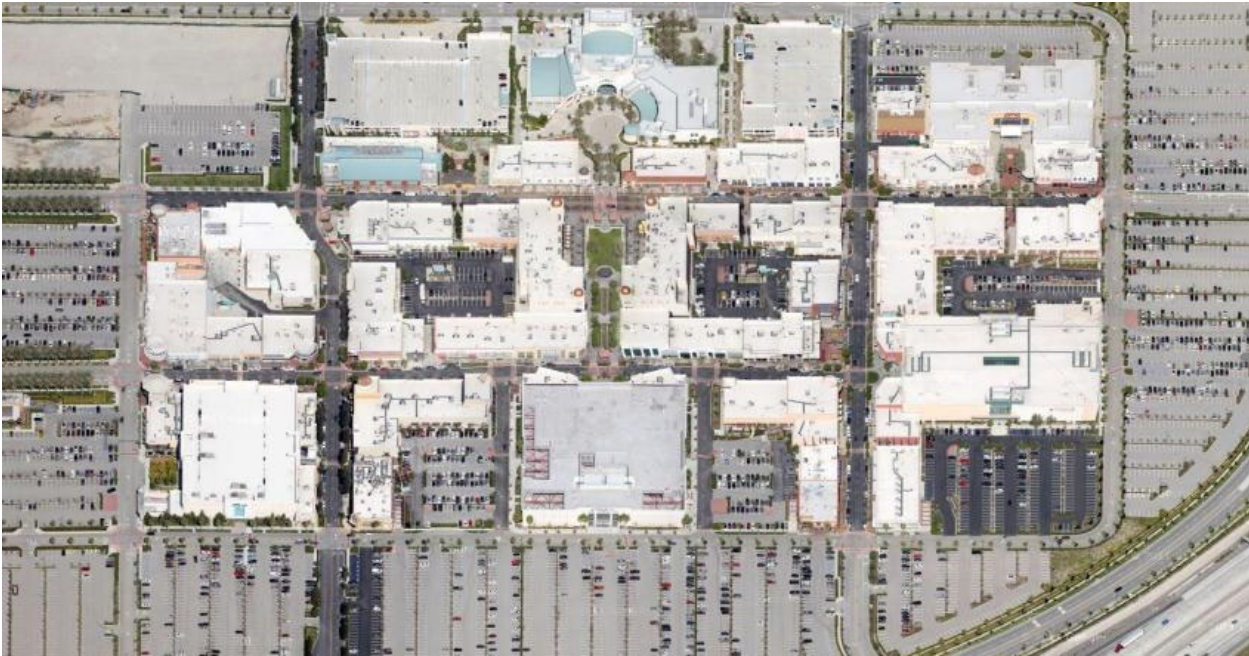
Vast parking lots are necessary to serve regional retailers but facades can still front onto internal streets rather than the lots.
