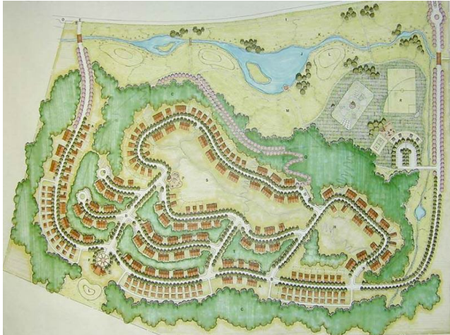
Cluster pattern achieved through “conservation subdivision” design (Source: University of Idaho Junior Design Studio).
