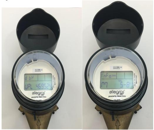
After approx. 10 gallons of water has run through the meter, the display will show the current reading.
