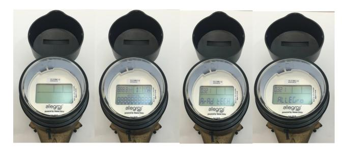
After the register has been activated and has scrolled through the four screens above, the register will toggle between the UPLINK frequency and the size the register is programmed for.
