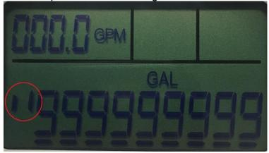
7.3 <u>Unit has made intial contact with the Base Station:</u> Unit has heard and connected to base station should have this indication.
