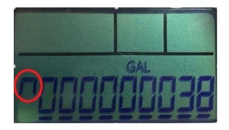
7.4 <u>Unit has synced with the Base Station:</u> Unit has fully connected to the base station.
