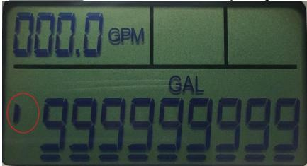
7.2 <u>Unit Not Synced with the Base Station:</u> The parallel lines indicate the register has not fully synced with the base station or repeater and is seeking.
