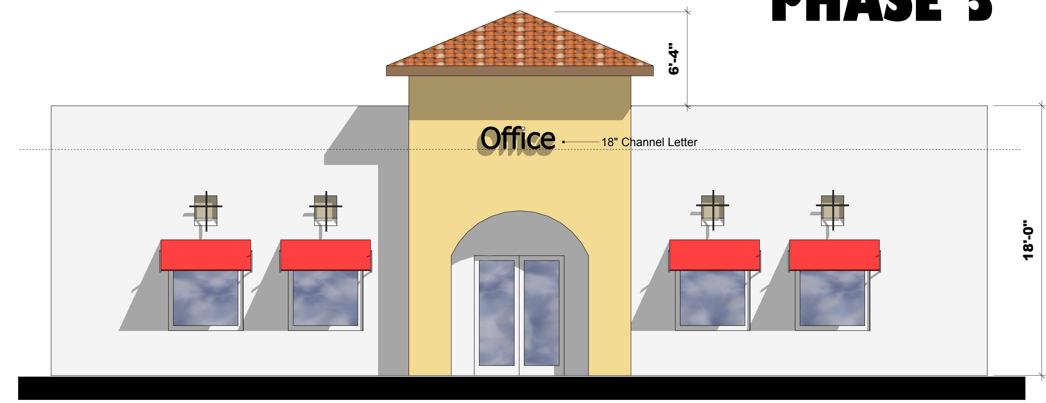
OFFICE FRONT ELEVATION Scale 1/4"=1'-0"
