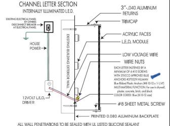
ALL WALL PENETRATIONS TO BE SEALED WITH UL LISTED SILICONE SEALANT U.L. 48
