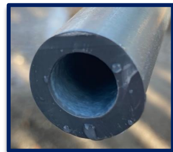
Figure 3. Cal Water Dixon Stannous Without Filtration Pilot Pipe with Chromium and Tin Accumulation.
