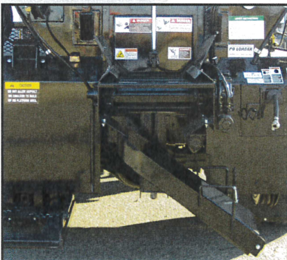
Pivoting Asphalt Chute
