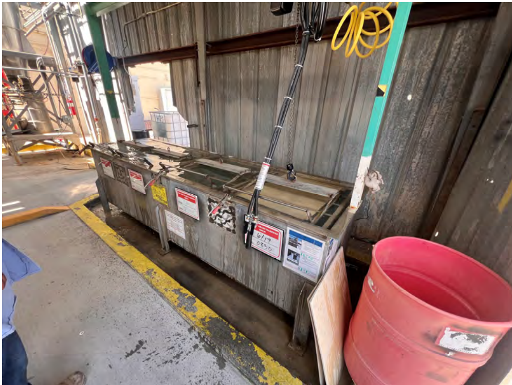
6. Typical view of a mold soak tank located in the exterior portion of Buildings 3, 6, and 9.
