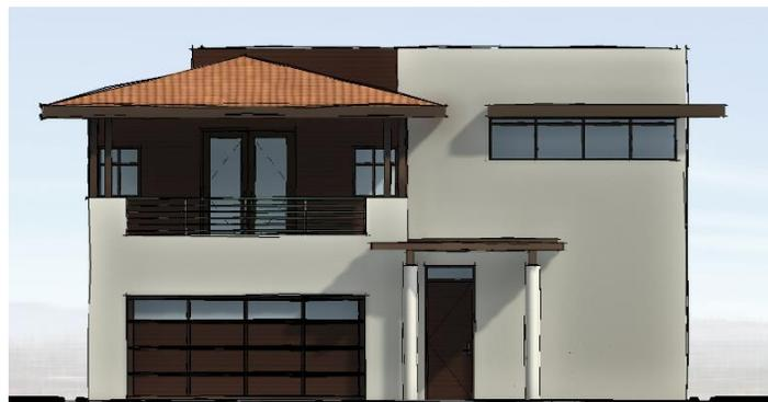
Plan D exterior building materials include stucco, garage door windows, second floor covered deck, concrete tile roof, covered entry, and long horizontal patterned windows. The roof pattern is a combination flat roof and hip roof design.
