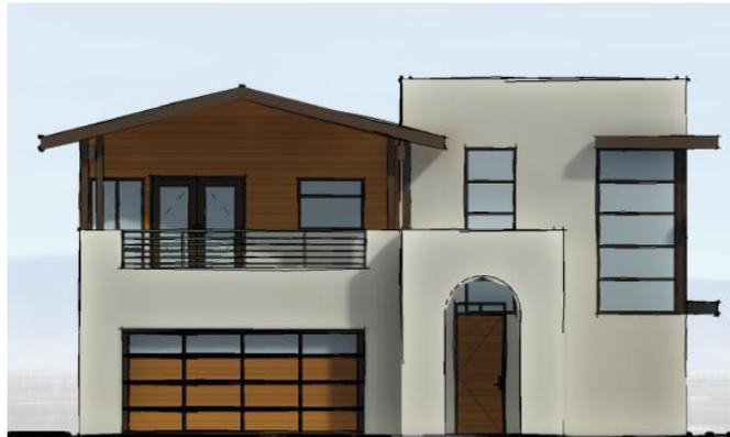
Plan B exterior materials include stucco, concrete tile roofing, second floor covered deck, garage door windows, large corner vertical window element, and covered entry. The roof includes gable and flat roof features.
