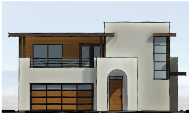
Plan C exterior building materials include stucco, garage door windows, second floor covered deck, covered entry. The roof pattern is a flat roof design.
