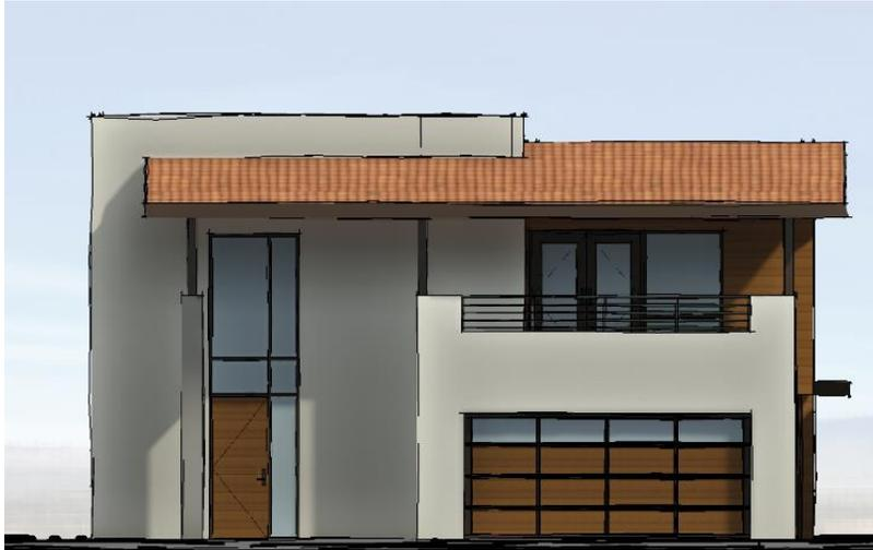
Plan E exterior building materials include stucco, garage door windows, concrete tile roof, second covered floor deck, covered entry, and long vertical patterned windows. The roof pattern is a combination flat roof and gable roof design.
