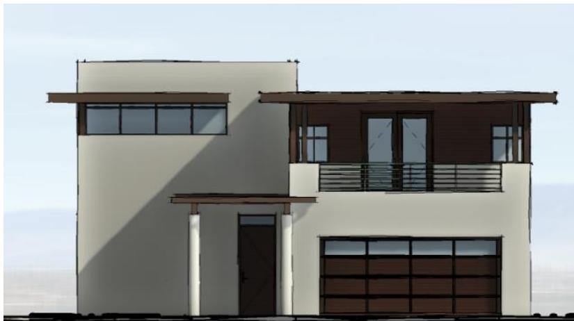
The Plan A exterior elevation includes exterior materials include stucco, flat roof, second floor covered deck, window garage doors, stucco projection at front corners, scored stucco accents, and covered entry.
