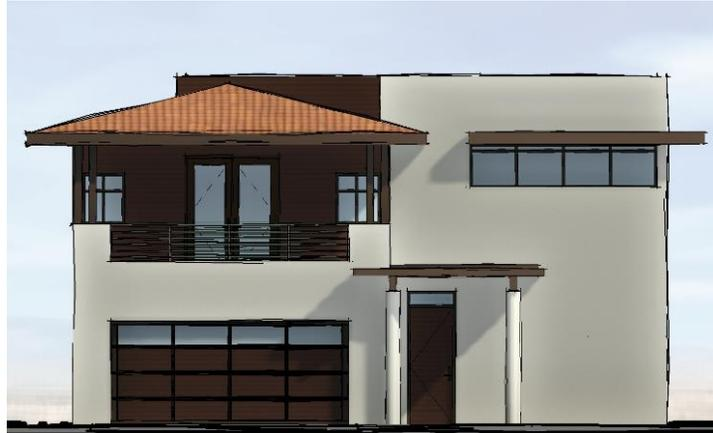
Plan G exterior building materials include stucco, garage door windows, second floor covered deck, covered entry, and long horizontal patterned windows. The roof pattern is a combination hip roof and flat roof design. Plan G is similar in appearance to Plan D.
