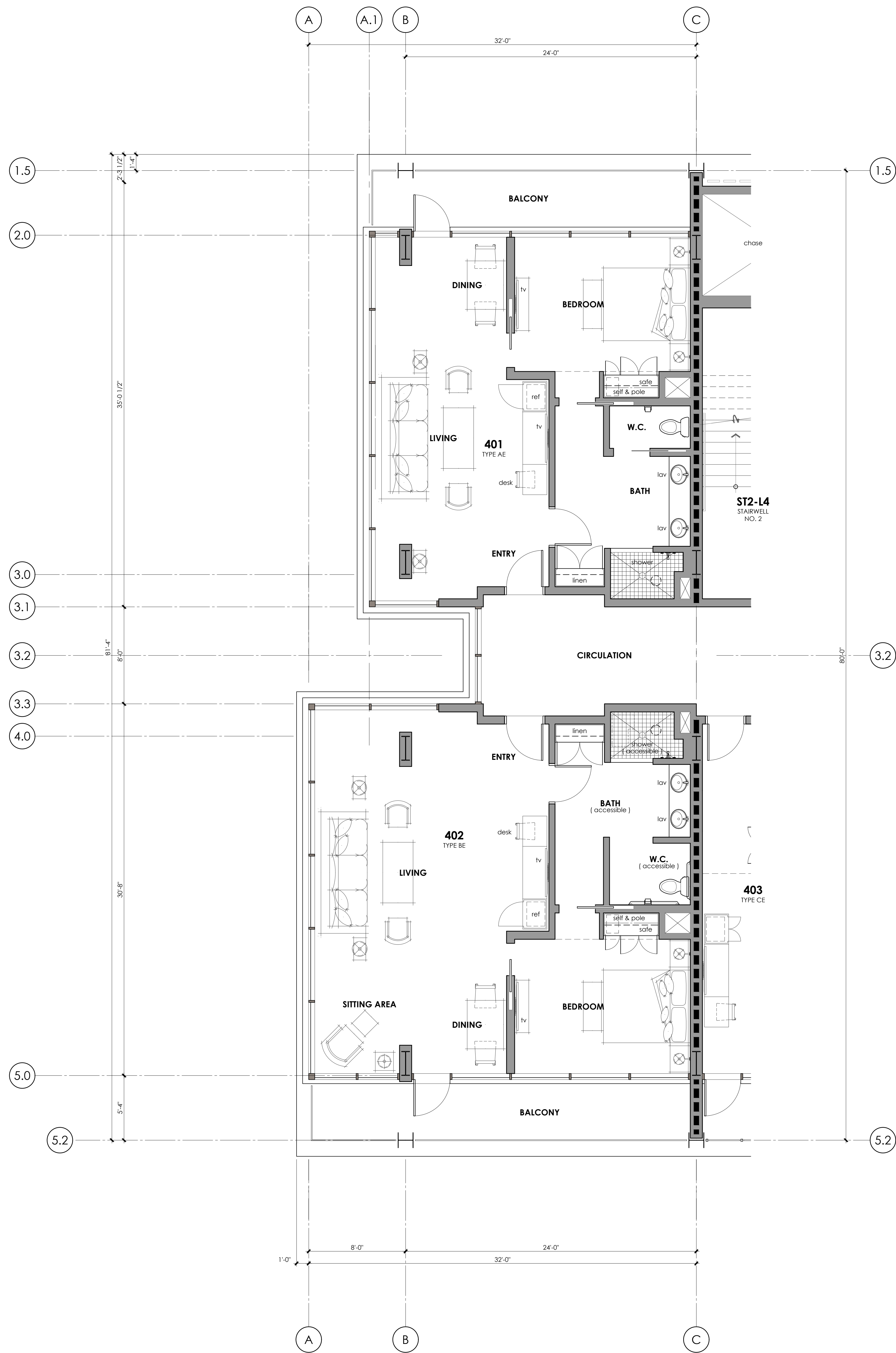
LEVEL 4 - SUITE 1 North - West Balcony Floor Plan with Optional Door To Bath scale : 1/4" = 1'-0"
