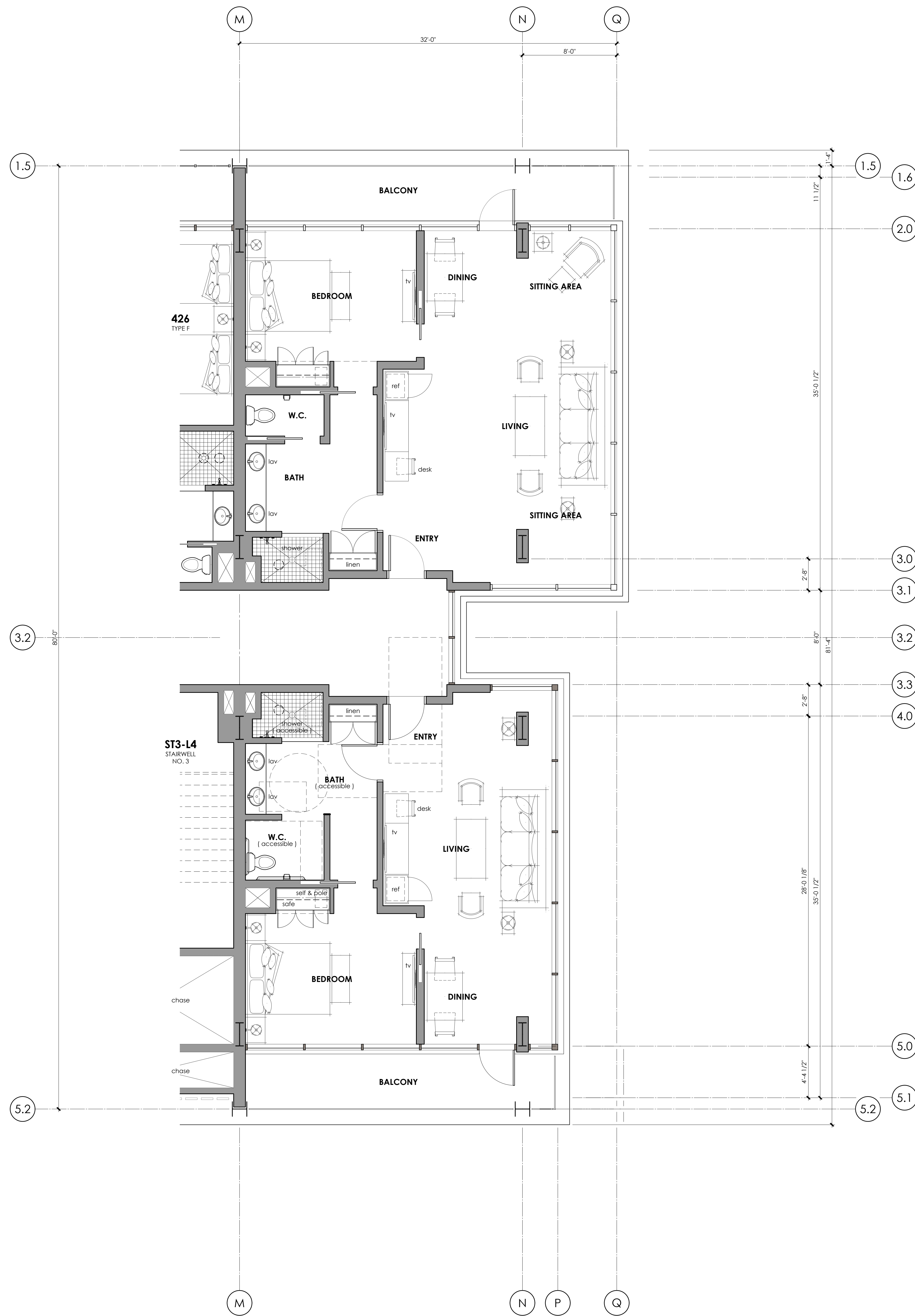
LEVEL 4 - SUITE 2 North - East Balcony Floor Plan with Optional Door To Bath scale : 1/4" = 1'-0"
