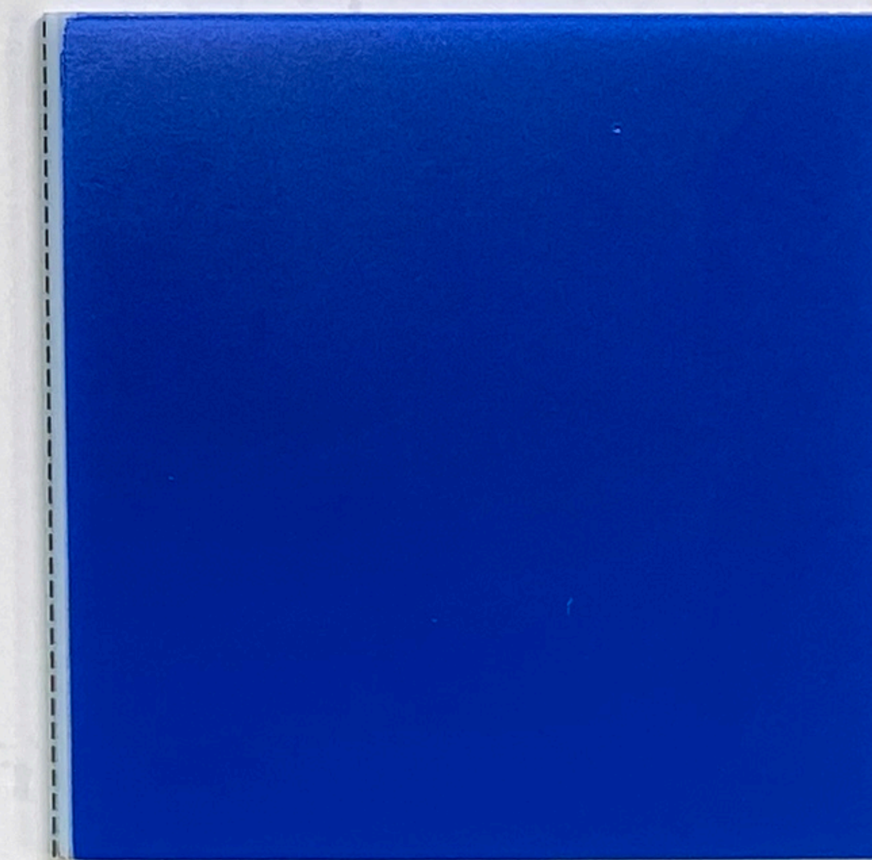
SIGN "B": • 3/16" THK. WHITE 7328 ACRYLIC UNDERLAY COPY • 3M BRIGHT BLUE #3630-167 TRANSLUCENT VINYL FILM
