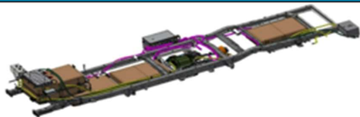
E450 FORD Chassis with EV system and batteries
