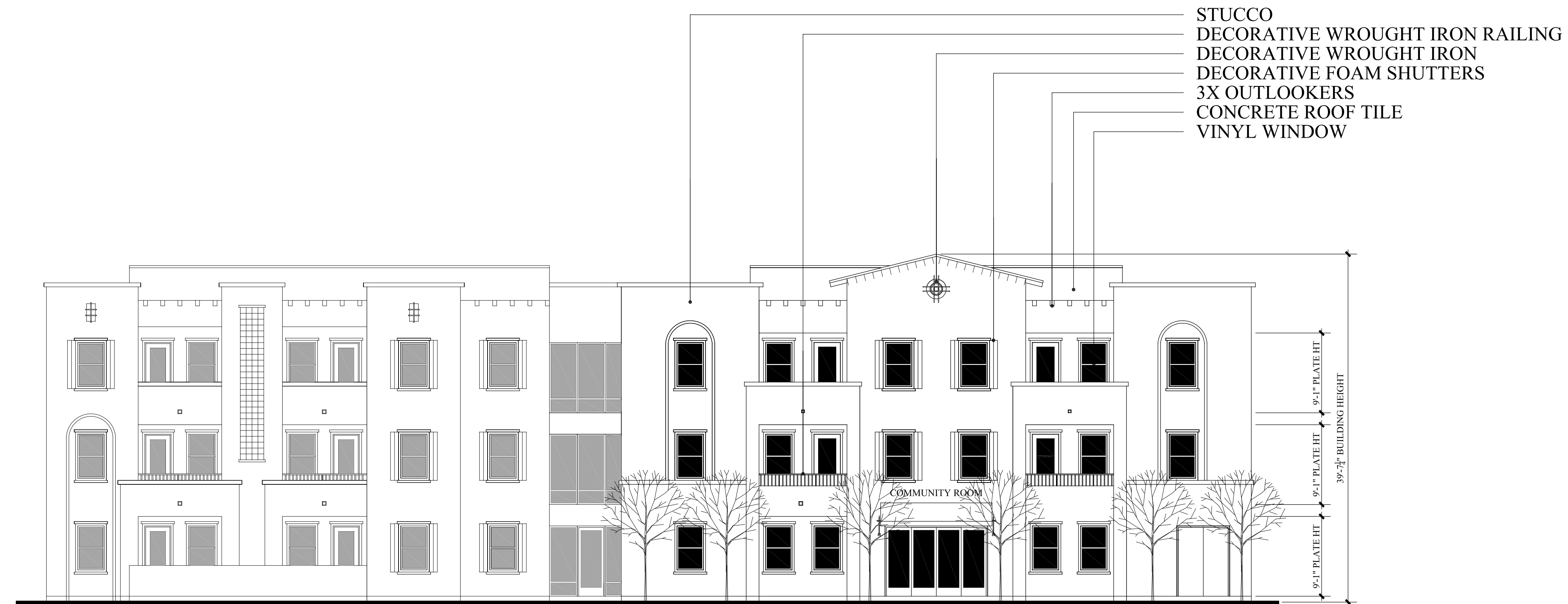
BUILDING A - SOUTH ELEVATION
