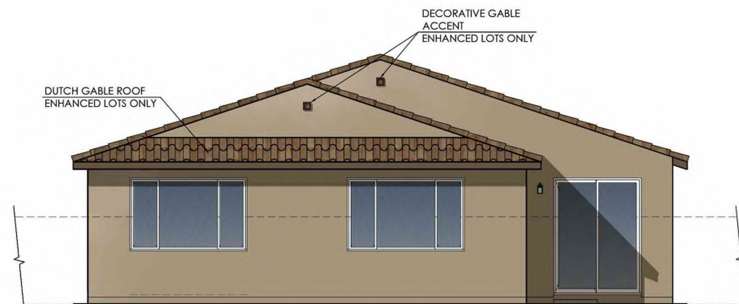
Rear Elevation "Enhanced"
