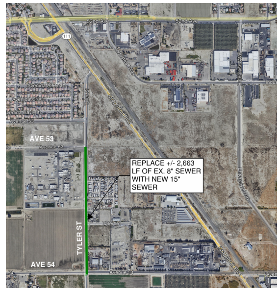
Figure 1: Sewer Replacement Location
