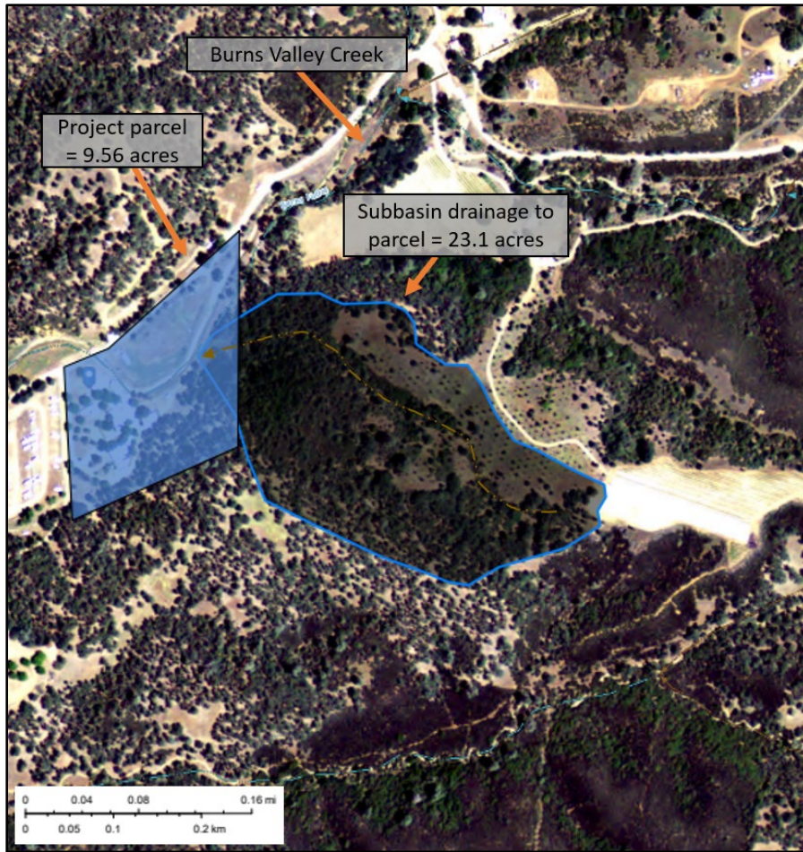
Figure 3: The recharge area for the proposed project is a 23.1-acre subbasin that drains to the project parcel and Burns Valley Creek.
