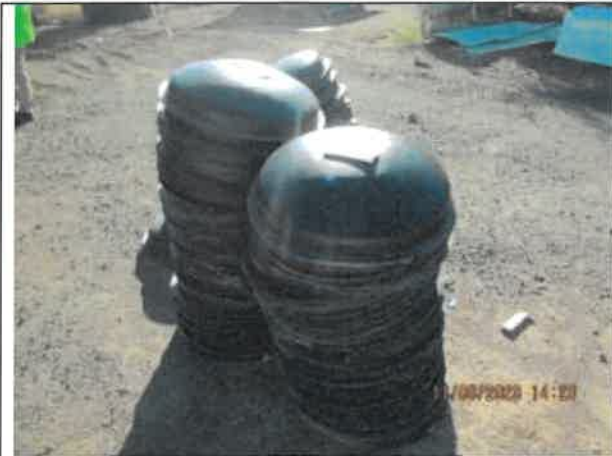
Photo 34: A photo of spare manhole barrier lids at the utility yard.
