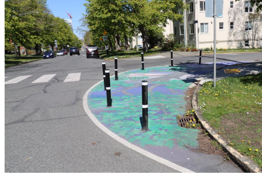
Example of a curb extension with vertical elements
