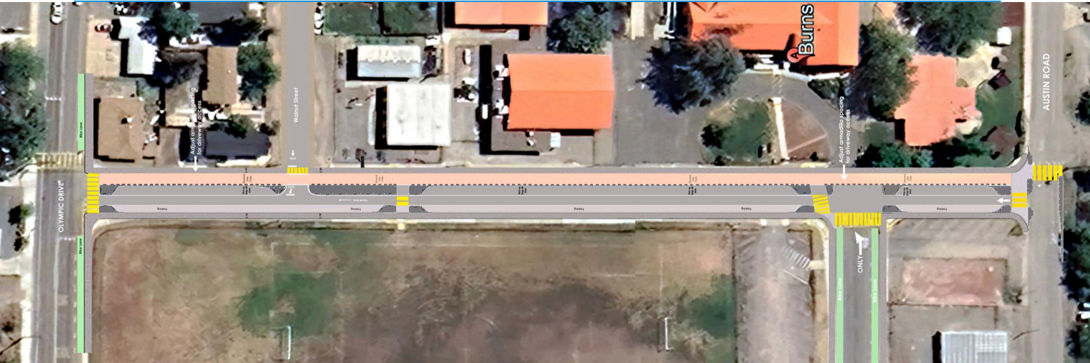
Image: Plan view of Pine Street showing conceptual layout of lanes, curb extensions, and pavement markings.
