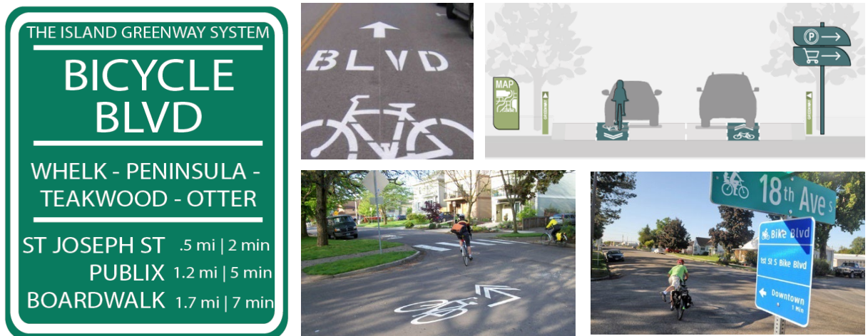
Photo and graphic examples of wayfinding signage and various enhanced shared lane markings.
