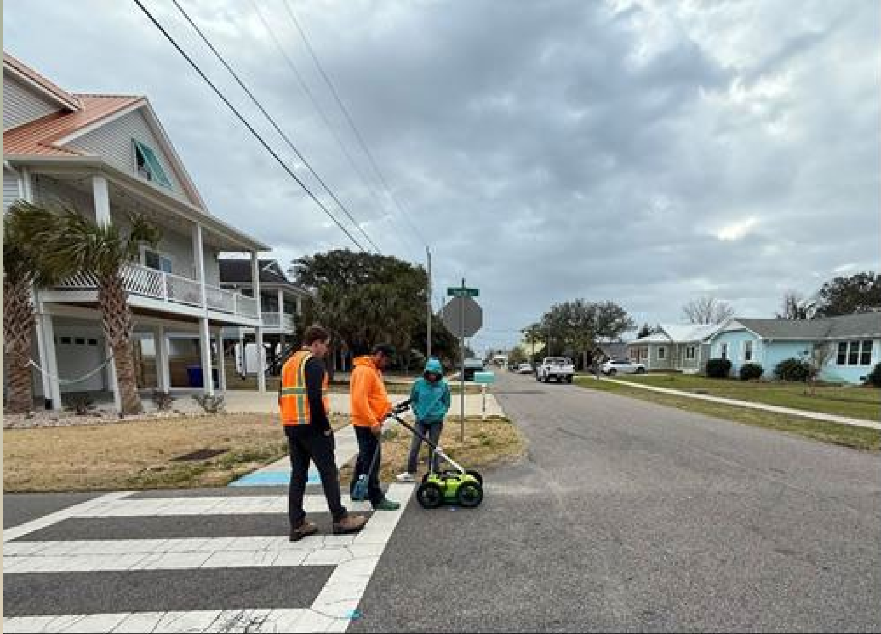
Staff worked with Jacobs Engineering on locating Town assets using Ground Penetrating Radar as part of AIA Grant
