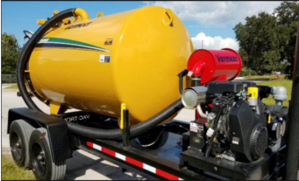
Figure 3: Vacuum with 800 gallon capacity tank to collect excess soil material
