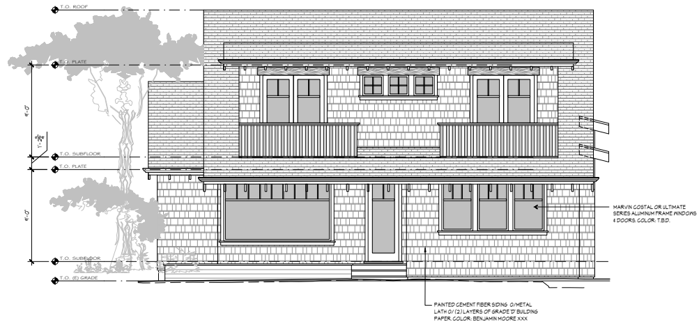
1 PROPOSED FRONT (SOUTH) ELEVATION SCALE: 1/4" = 1'-0"
