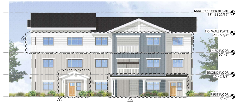
BUILDING D - WEST ELEVATION | 1/8" = 1'-0" | 4
