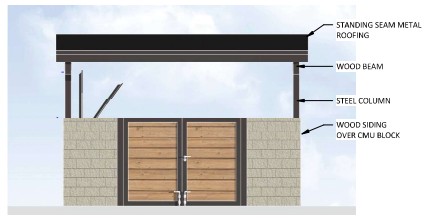
FRONT ELEVATION | 1/4" = 1'-0" | 1/A2.11 | 6
