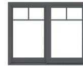
7. VINYL WINDOW FRAMES COLOR: CHARCOAL GRAY FROM MANUFACTURER'S STANDARD COLORS
