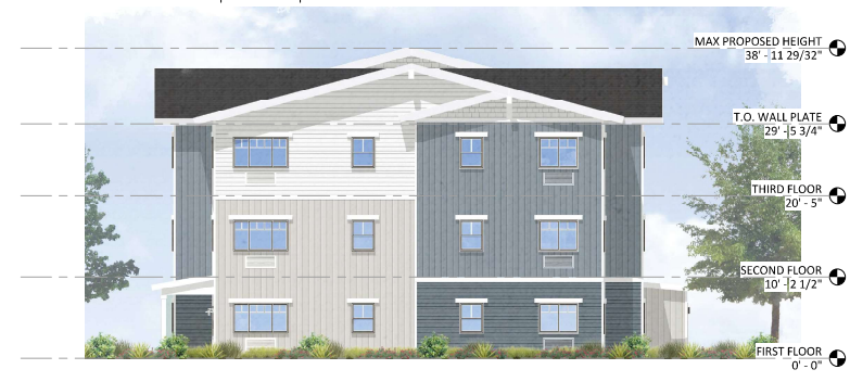
BUILDING D - SOUTH ELEVATION | 1/8" = 1'-0" | 1
