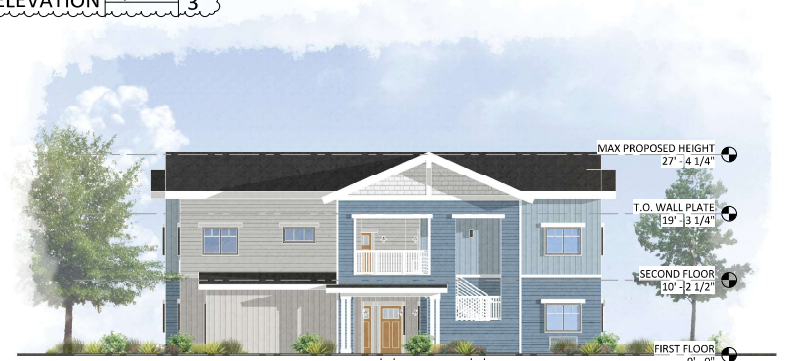
BUILDING A - EAST ELEVATION 1/8" = 1'-0" 2
