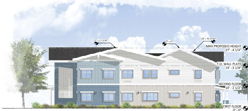
BUILDING A - NORTH ELEVATION 1/8" = 1'-0" 3
