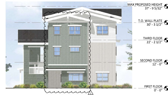
BUILDING B - EAST ELEVATION | 1/8" = 1'-0" | 2
