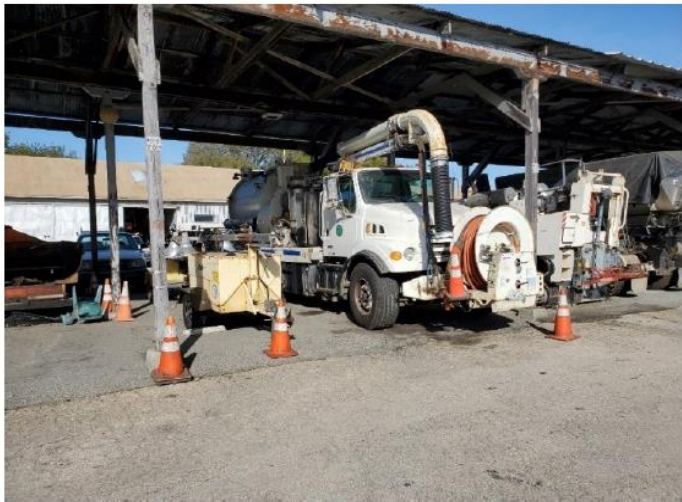
Figure 2. Vactor Truck at Brommer Yard
