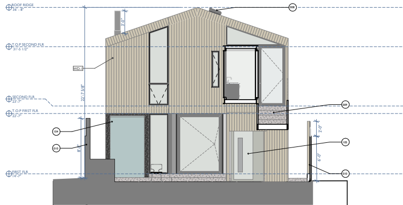
1 PROPOSED RESIDENCE EAST COURTYARD ELEVATION SCALE: 1/4" = 1'-0"
