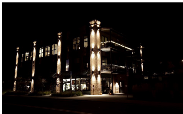
Figure 103. Example of architectural lighting that draws attention to unique architecture, in this case the simple columns of the building, making it stand out even at night. Apartment building, Duluth, MN. [Photo credit: Seanette Corkill]
