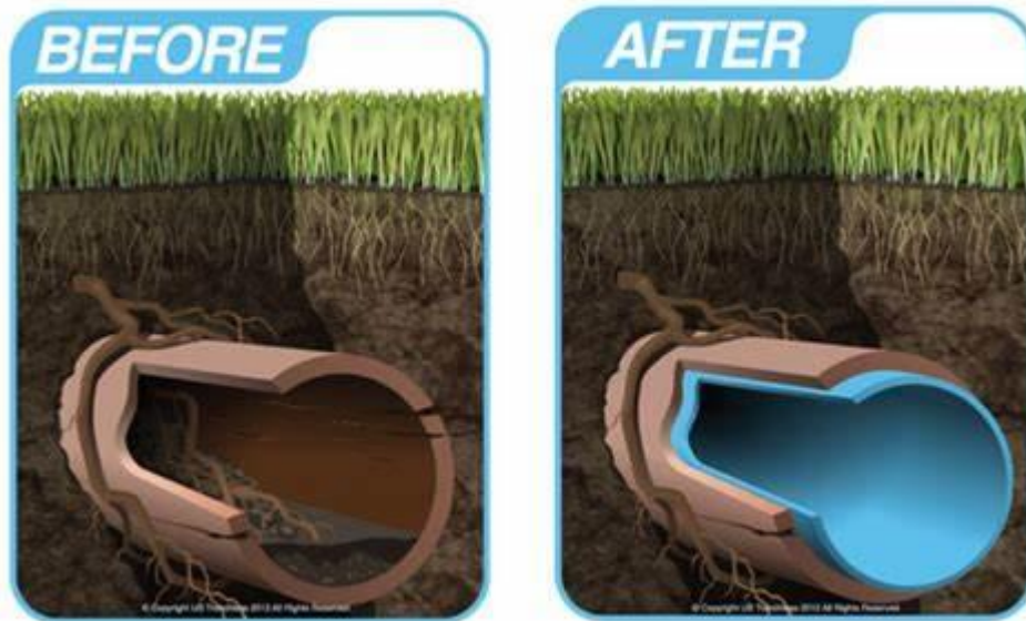
Figure 2. Illustration of before and after CIPP
