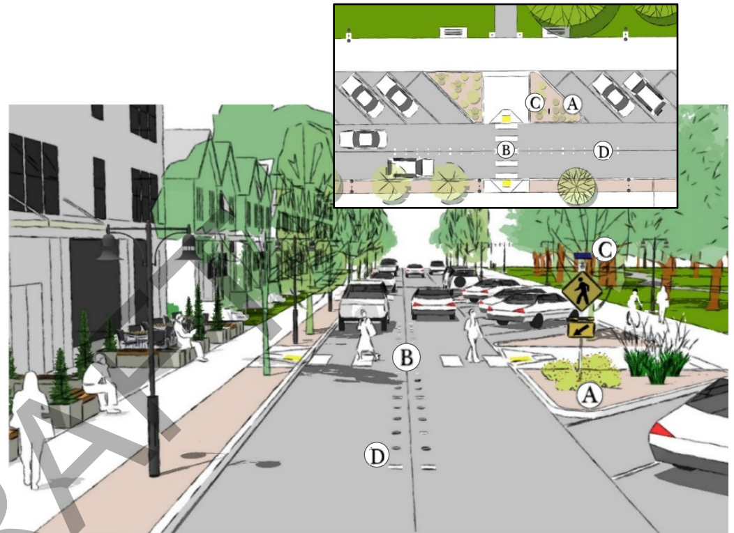
Figure 15. Enhanced crossing elements
