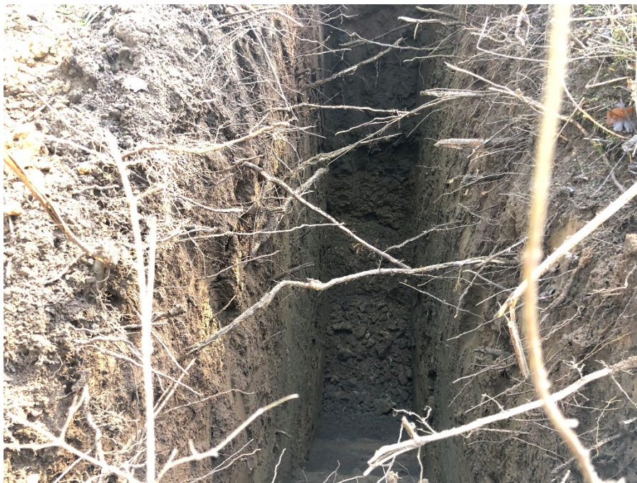
Medium-Sized Roots within Test Pit TP-6
