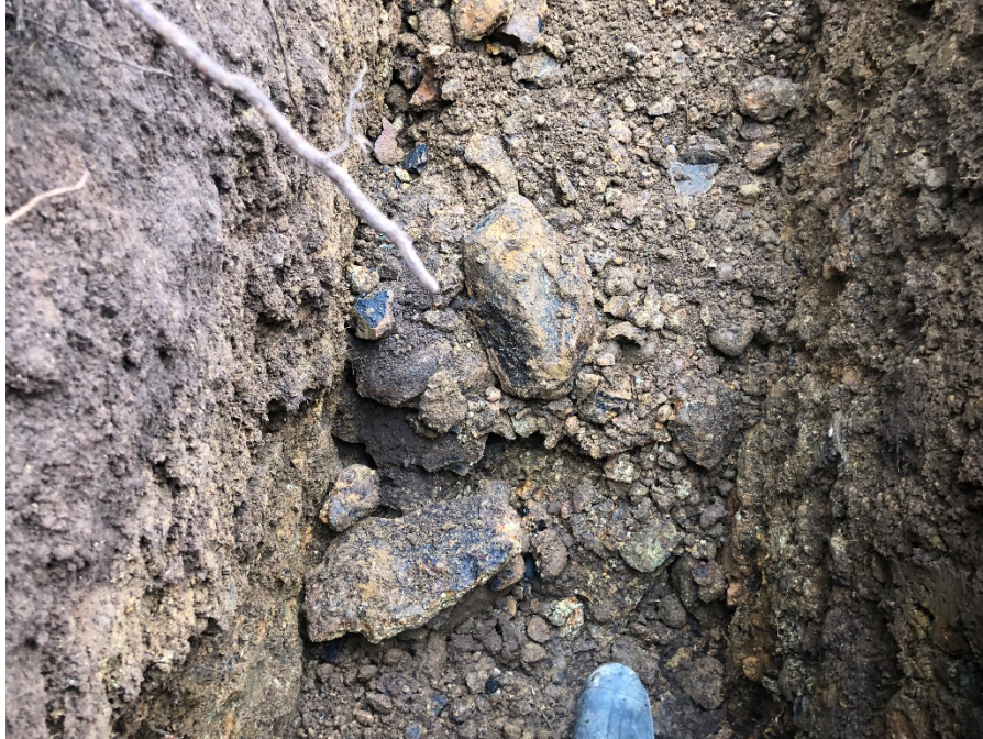
Dense Conglomerate in Test Pit TP-8
