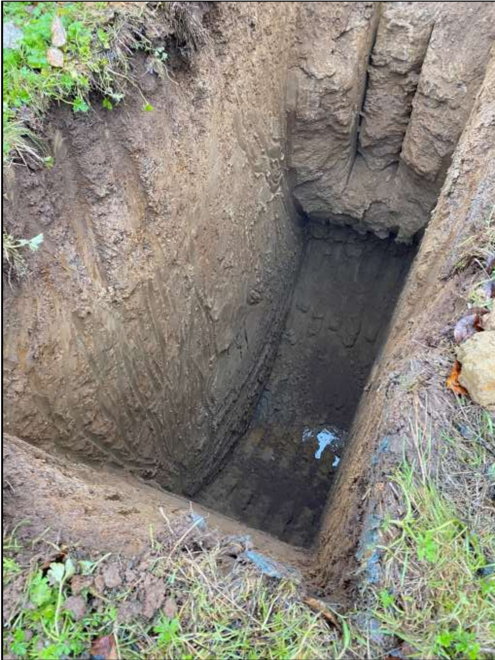
Typical Test Pit Profile, TP-4
