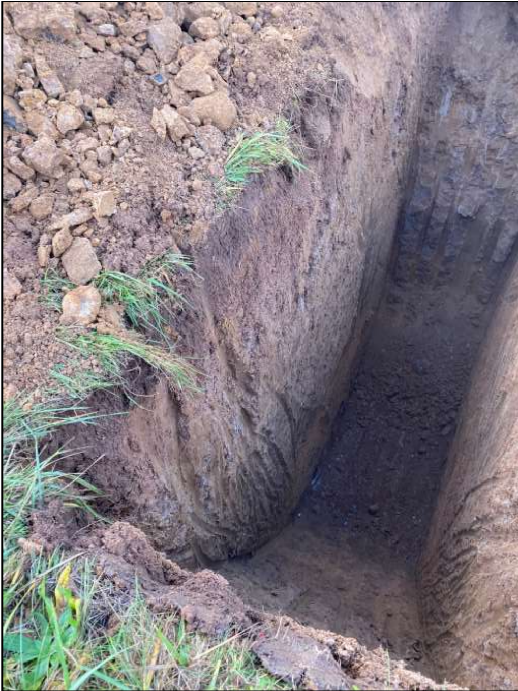
Typical Test Pit Profile, TP-1
